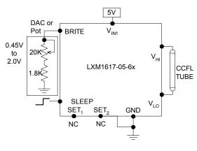
Figure 1 – Brightness Control (output current set to maximum)
