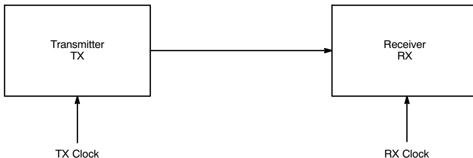
Figure 33. Example of a Serial Data Transmission System
