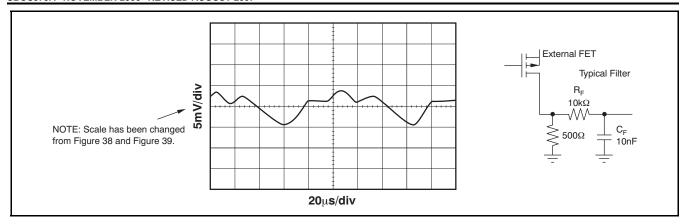
Figure 41. Output with Additional Filter
