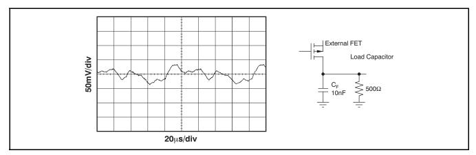
Figure 40. Output with 10nF Parallel to 500 $\Omega$
