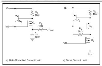
Figure 37. External Current Limit Circuits
