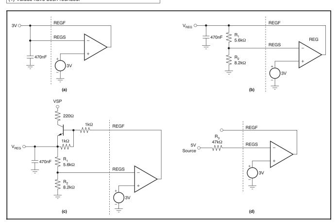
Figure 45. Basic Connections of the Voltage Regulator
