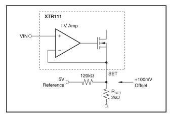
Figure 44. Input Voltage Level Shift for 0mA
