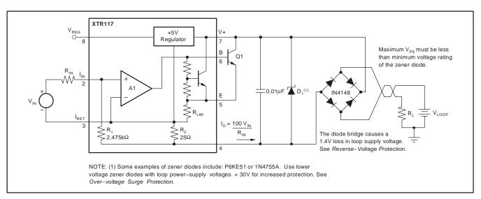
Figure 3. Reverse Voltage Operation and Over-Voltage Surge Protection
