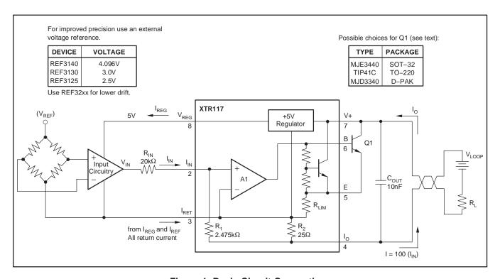
Figure 1. Basic Circuit Connections
