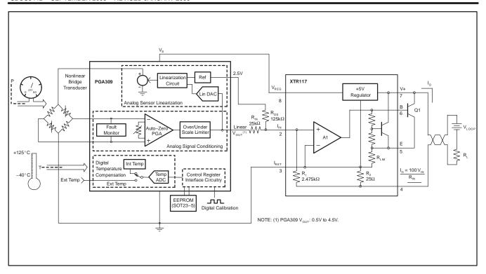
Figure 5. Complete 4-20mA Pressure Transducer Solution with PGA309 and XTR117
