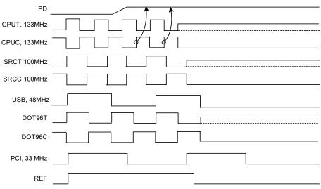
Figure 3. Power-down Assertion Timing Waveform
