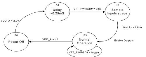
Figure 6. Clock Generator Power-up/Run State Diagram
