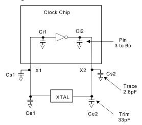
Figure 2. Crystal Loading Example
