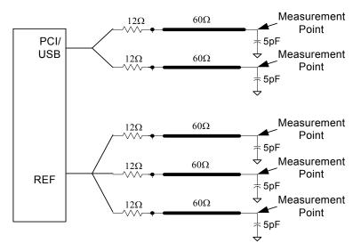
Figure 7. Single-ended Load Configuration
