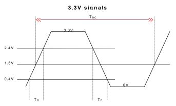
Figure 9. Single-ended Output Signals (for AC Parameters Measurement)
