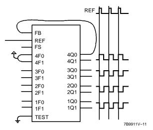
**Figure 4. Inverted Output Connections**
