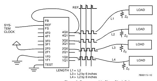
Figure 3. Programmable-Skew Clock Driver
