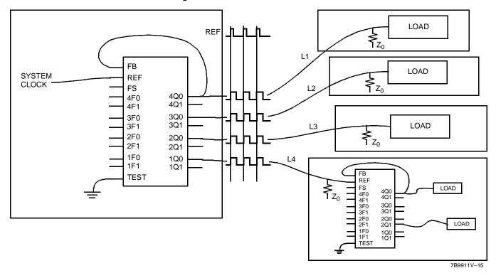
Figure 8. Board-to-Board Clock Distribution
