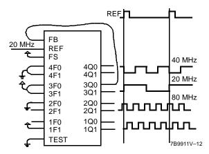
Figure 5. Frequency Multiplier with Skew Connections
