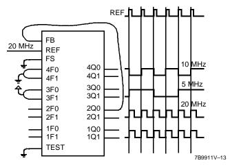
Figure 6. Frequency Divider Connections
