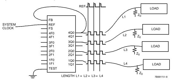
Figure 2. Zero-Skew and/or Zero-Delay Clock Driver
