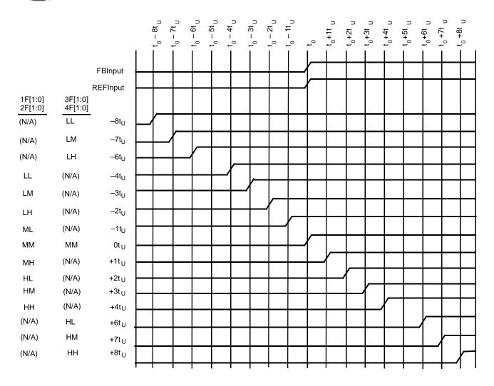
Figure 1. Typical Outputs with FB Connected to a Zero-Skew Output<sup>[4]</sup>
