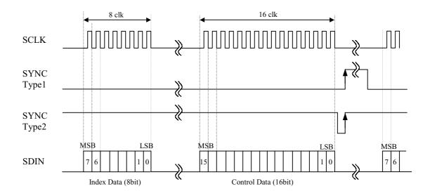
The YMU757B is controlled through the three serial interfaces SCLK, SYNC and SDIN.
