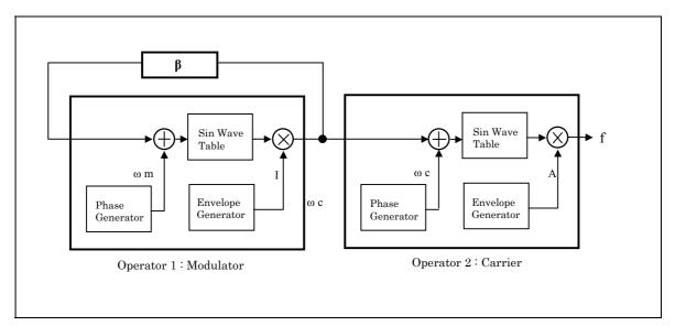
The "Operator" refers to the section where a sine wave is generated and the combination of the operators is called "algorithm". The operator in the front stage is called "modulator" and that in the rear stage "carrier".
