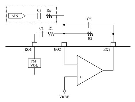
Gain and filter characteristic are adjusted by value of C1, C2, R1 and R2. Gain = R2 / R1. Recommendation of R1 is  $22k\Omega$  and R2 is  $82k\Omega$  (gain = 3.7 times). Cut off frequency f1 and f2 of filter is as follows.
