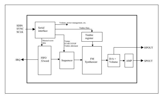
When the data is inputted into the serial interface, it is converted into the parallel data and transmitted to each function block according to the index address.
