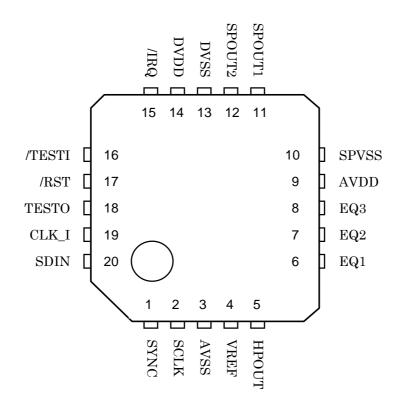
20 Pin QFN Top View
