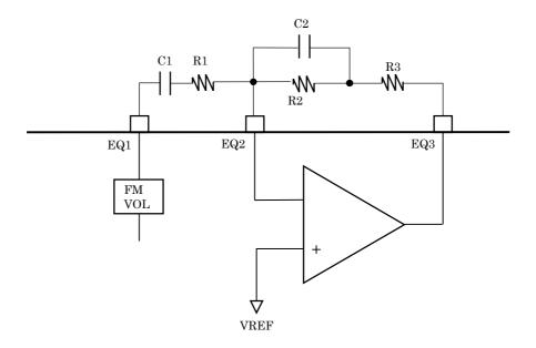
Gain1= (R2+R3) /R1. Gain2=R3/R1. Cut off frequency f1 and f2 of filter is as follows.
