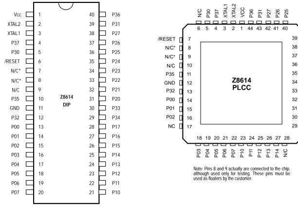
Note: Pins 7 and 8 actually are connected to the chip, although used only for testing. These pins must be used as floaters by the customer.
