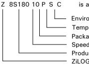
is a Z8S180 10-MHz 60-Pin DIP, 0° to +70°C, Plastic Standard Flow
