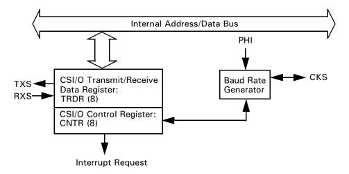
Figure 7. CSI/O Block Diagram
