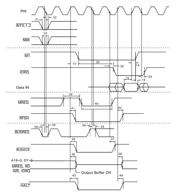
Figure 21. CPU Timing (INTO Acknowledge Cycle, Refresh Cycle, BUS RELEASE Mode, HALT Mode, SLEEP Mode, SYSTEM STOP Mode)
