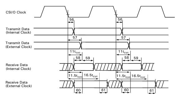
Figure 29. CSI/O Receive/Transmit Timing
