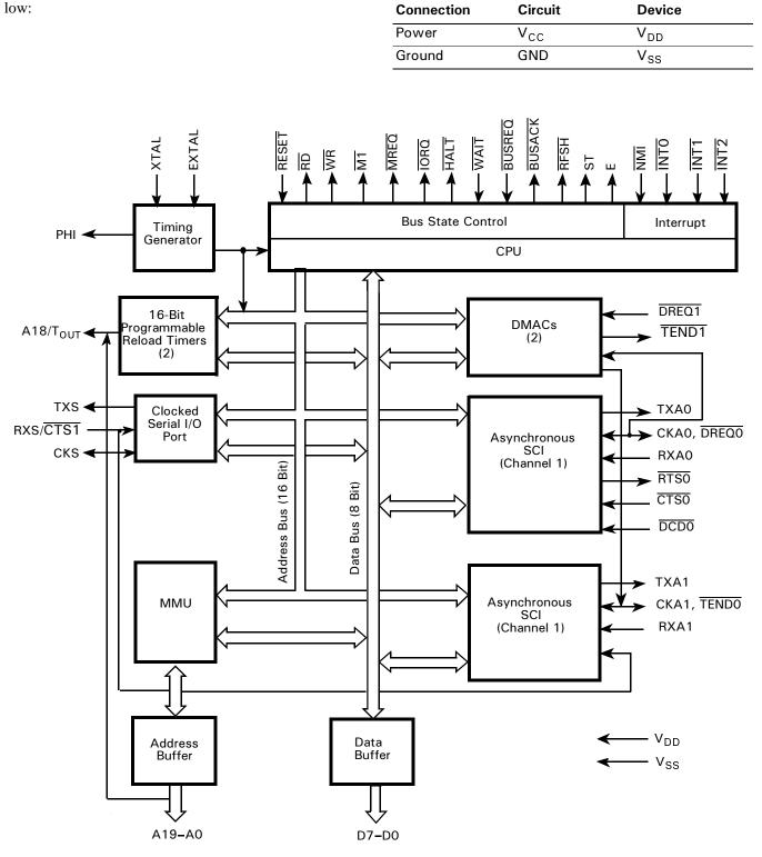
Figure 1. Z8S180/Z8L180 Functional Block Diagram
