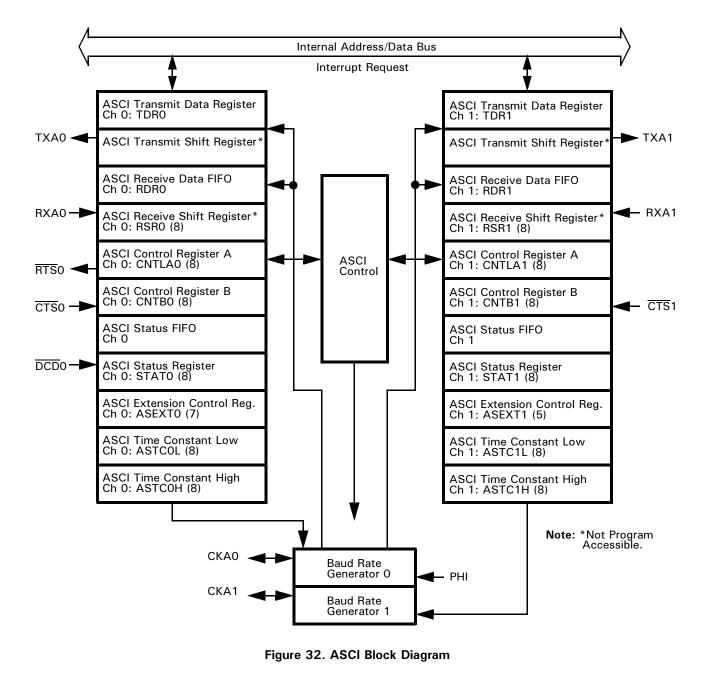
**ASCI Transmit Shift Register 0,1.** When the ASCI Transmit Shift Register (TSR) receives data from the ASCI Transmit Data Register (TDR), the data is shifted out to the TXA pin. When transmission is completed, the next byte (if available) is automatically loaded from TDR into TSR and the next transmission starts. If no data is available for trans-
