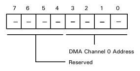
Figure 57. DMA Source Address Register 0B
