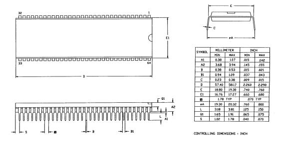
Figure 85. 64-Pin DIP Package Diagram
