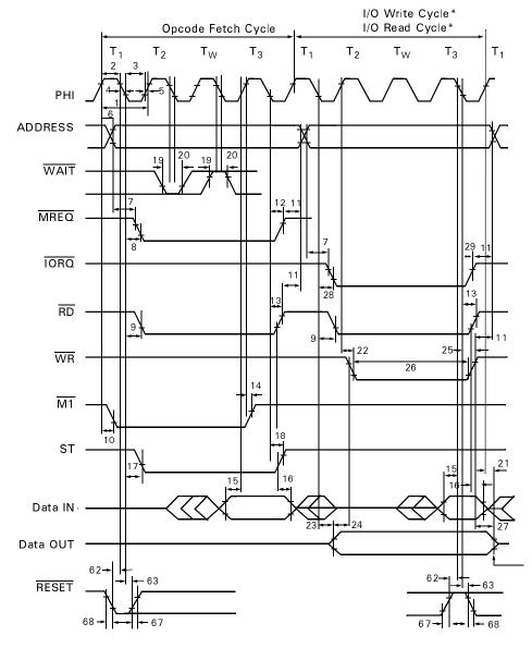
Note: \*Memory Read/Write Cycle timing is the same as I/O Read/Write Cycle except there are no automatic wait states ( $T_W$ ), and  $\overline{MREQ}$  is active instead of  $\overline{IORQ}$ .
