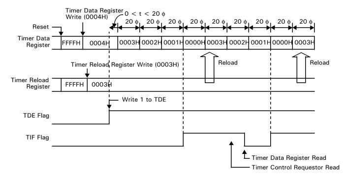
Figure 5. Timer Initialization, Count Down, and Reload Timing
