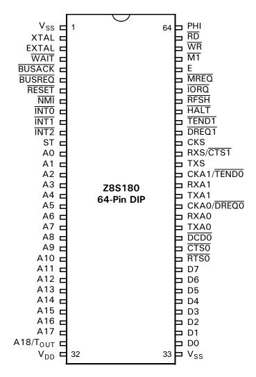
Figure 2. Z8S180 64-Pin DIP Pin Configuration
