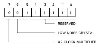
Figure 54. Clock Multiplier Register
