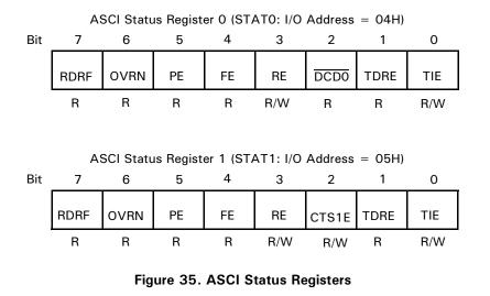
**RDRF: Receive Data Register Full (Bit 7).** RDRF is set to 1 when an incoming data byte is loaded into an empty Rx FIFO. If a framing or parity error occurs, RDRF is still set and the receive data (which generated the error) is still loaded into the FIFO. RDRF is cleared to 0 by reading RDR and most recently received character in the FIFO from IOSTOP mode, during RESET and for ASCI0 if the DCD0 input is auto-enabled and is negated (High).
