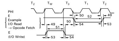
Figure 26. E Clock Timing (Minimum Timing Example of  $P_{\text{WEL}}$  and  $P_{\text{WEH}}$ )
