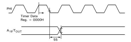
Figure 27. Timer Output Timing
