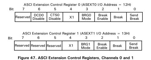
**DCD0 Disable (Bit 6, ASCIO Only).** If this bit is 0, then the  $\overline{DCD0}$  pin auto-enables the ASCI0 receiver, such that when the pin is negated/High, the Receiver is held in a RE-SET state. If this bit is 1, the state of the  $\overline{DCD}$ -pin has no effect on receiver operation. In either state of this bit, software can read the state of the  $\overline{DCD0}$  pin in the STAT0 register, and the receiver interrupts on a rising edge of  $\overline{DCD0}$ .
