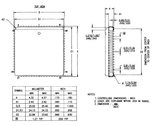
Figure 87. 68-Pin PLCC Package Diagram
