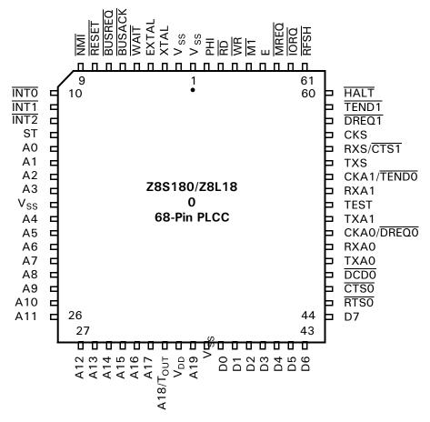
Figure 3. Z8S180/Z8L180 68-Pin PLCC Pin Configuration
