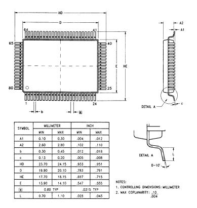
Figure 86. 80-Pin QFP Package Diagram
