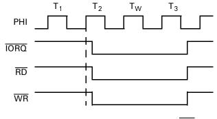
Figure 12. I/O Read and Write Cycles with  $\overline{IOC} = 0$
