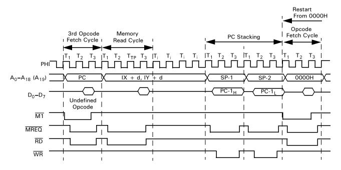
Figure 76. TRAP Timing-3<sup>rd</sup> Opcode Undefined
