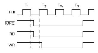
Figure 11. I/O Read and Write Cycles with  $\overline{IOC} = 1$
