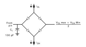
Figure 19. AC Parameter Test Circuit
