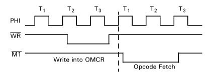
Figure 10. M1 Temporary Enable Timing
