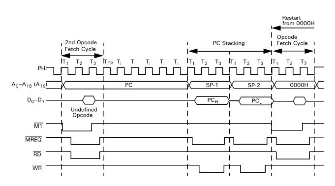
Figure 75. TRAP Timing—2<sup>nd</sup> Opcode Undefined
