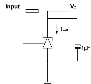
Fig 3 – Test Circuit for Off State current
