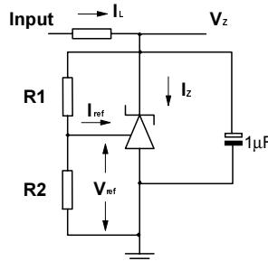
Fig 2 – Test Circuit for  $V_z > V_{ref}$
