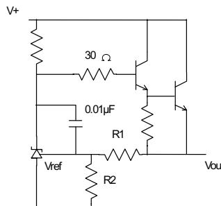
$$V_{out} = \left(1 + \frac{R_1}{R_2}\right) V_{ref}$$
