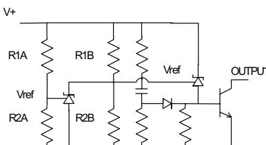
$$\text{Low limit} = \left(1 + \frac{R_1B}{R_2B}\right) V_{ref}$$
