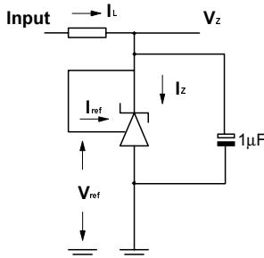
Fig 1 – Test Circuit for  $V_z = V_{ref}$
