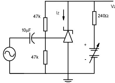
$I_Z = 10\text{mA}, TA = 25^\circ\text{C}$
