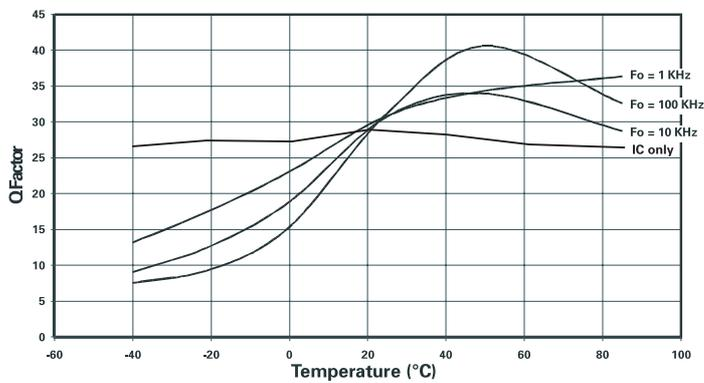
Components used: 1/8 watt metal film resistors ( $\pm 50$  ppm). Ceramic capacitors ( $\pm 50$  ppm).
