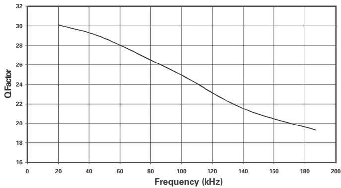
The curve shows Q Factor over frequency for a fixed loop gain ( $R_f/R_i$ ).
