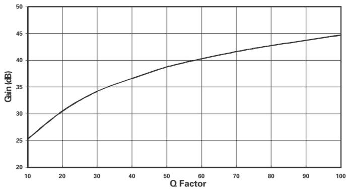
Gain at  $f_o$  describes the peak gain of the notch pass filter. This gain is defined by the value of Q Factor.
