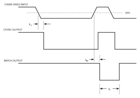
Figure 3: SYNC SLICING & OUTPUT DETAIL
