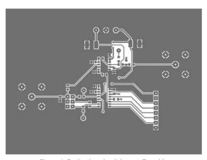
Figure 6: Evaluation circuit layout: Top side
