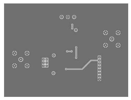
Figure 7: Evaluation circuit layout: Bottom side (viewed through board)
