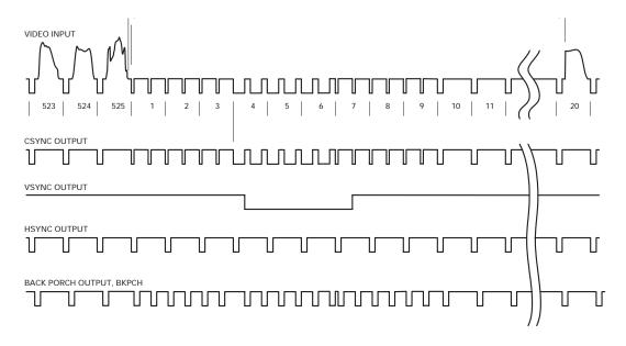
Figure 2: NTSC TIMING DIAGRAM
