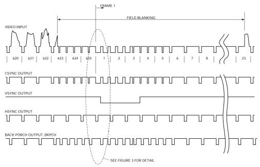
Figure 1: PAL 625 TIMING DIAGRAM
