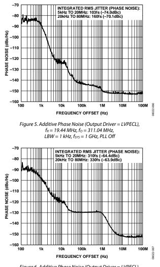
Figure 6. Additive Phase Noise (Output Driver = LVPECL),  $f_R = 19.44$  MHz,  $f_0 = 311.04$  MHz, LBW = 1 kHz,  $f_{SYS} = 50$  MHz (Crystal), PLL On
