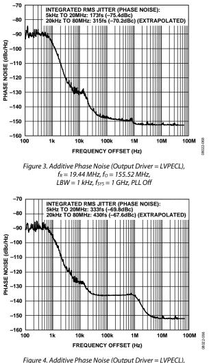
fgure 4. Additive Phase Noise (Output Driver = LVPE  $f_R = 19.44 \text{ MHz}, f_0 = 155.52 \text{ MHz},$  $LBW = 1 \text{ kHz}, f_{SYS} = 50 \text{ MHz}$  (Crystal), PLL On
