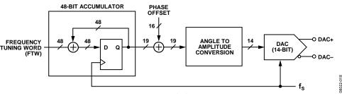
Figure 42. DDS Block Diagram
