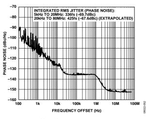
Figure 9. Additive Phase Noise (Output Driver = LVPECL),  $f_R = 8 \text{ kHz}, f_O = 155.52 \text{ MHz},$  $LBW = 100 \text{ Hz}, f_{SYS} = 50 \text{ MHz}$  (Crystal), PLL On
