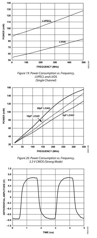
Figure 21. Output Waveform, LVPECL (400 MHz)
