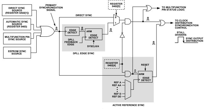
Figure 48. Output Synchronization Block Diagram
