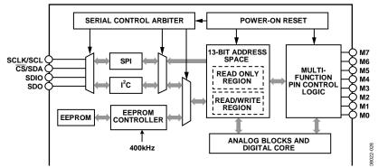
Figure 51. Serial Port Functional Diagram
