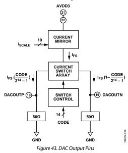
The value of  $I_{FS}$  is programmable via the 10-bit DAC full-scale current word in the DAC current register (Address 0213 to Address 0214). The value of the 10-bit word ( $I_{SCALE}$ ) sets  $I_{FS}$  according to the following formula:
