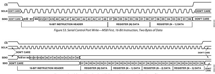
Figure 54. Serial Control Port Read—MSB First, 16-Bit Instruction, Four Bytes of Data
