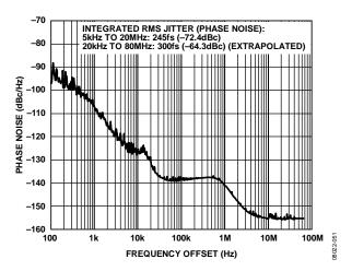
Figure 12. Additive Phase Noise (Output Driver = LVPECL),  $f_R = 19.44 \text{ MHz}, f_0 = 155.52 \text{ MHz},$   $LBW = 1 \text{ kHz}, f_{SYS} = 50 \text{ MHz}$  (Crystal), PLL On with 2x Frequency Multiplier,  $I_{CP} = 375 \mu$ A, LF = External (350 kHz)
