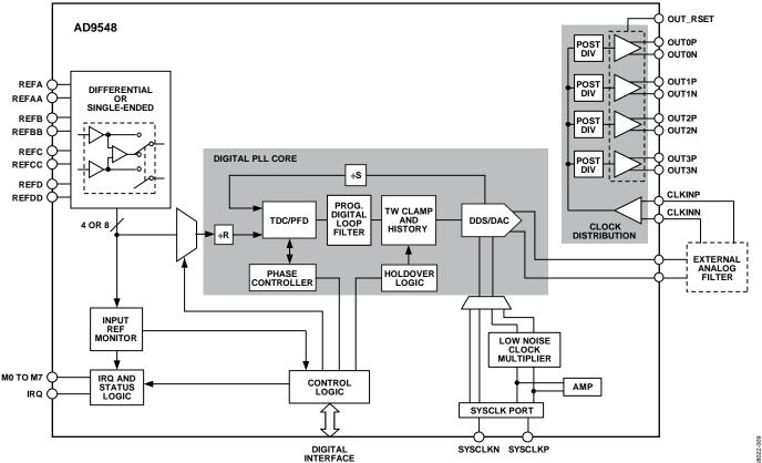
Figure 33. Detailed Block Diagram
