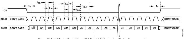
Figure 55. Serial Control Port Write—MSB First, 16-Bit Instruction, Timing Measurements
