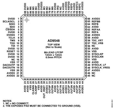
Figure 2. 88-Lead LFCSP Pin Configuration
