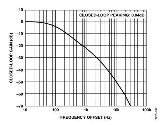
Figure 16. Jitter Transfer Bandwidth, Output Driver = LVPECL,  $f_R = 19.44 \text{ MHz}, f_O = 155.52 \text{ MHz},$ LBW = 100 Hz (Phase Margin = 88°),  $f_{SYS} = 1 \text{ GHz}, \text{PLL Off}$
