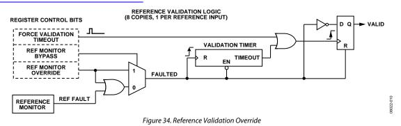
The main feature to note is that any time faulted = 1, the output latch is reset, which forces valid = 0 (indicating an invalid reference) regardless of the state of any other signal. Under the default condition (that is, all three control bits are 0), the reference monitor is the primary source of the validation process. This is because, under the default condition, the ref fault signal from the reference monitor is identically equal to the faulted signal.
