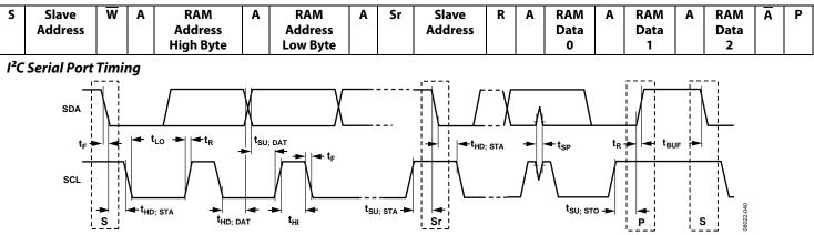
Figure 64. I<sup>2</sup>C Serial Port Timing
