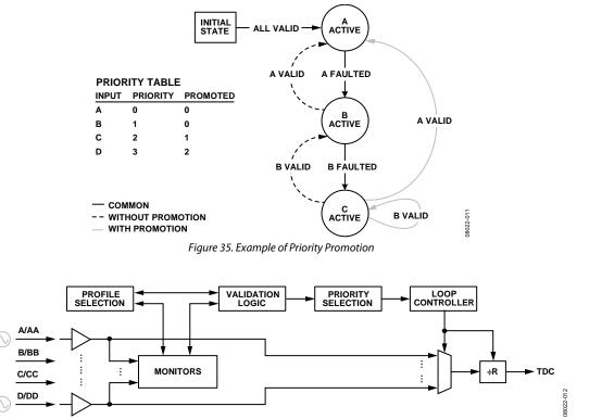
Figure 36. Reference Clock Block Diagram
