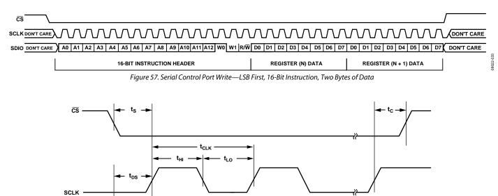
Figure 58. Serial Control Port Timing—Write
