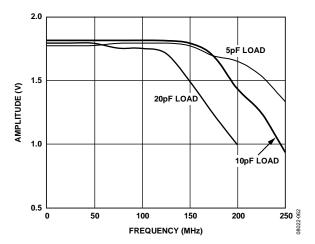
Figure 17. Amplitude vs. Toggle Rate, 1.8 V CMOS
