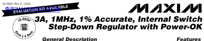
The MAX8505 step-down regulator operates from a 2.6V to 5.5V input and generates an adjustable output voltage from 0.8V to 0.85 × VIN at up to 3A. With a 2.6V to 5.5V bias supply, the input voltage can be as low as 2.25V.
