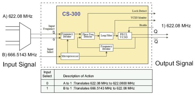
All components outside the dotted line box are user supplied components and/or connections. This is just one possible configuration of the CS-300. For additional information about your specific needs please contact our Factory.
