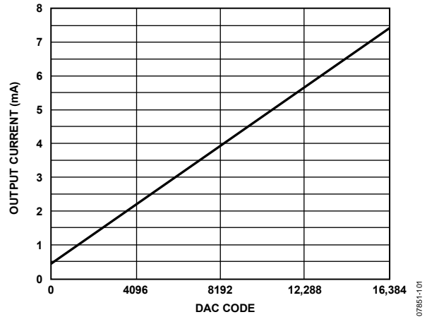
Figure 104. Gain Curve for FSC[9:0] = 0, DAC OFFSET = 0.257 mA
