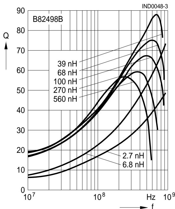
**Q factor versus frequency  $f$  (ferrite core)**
