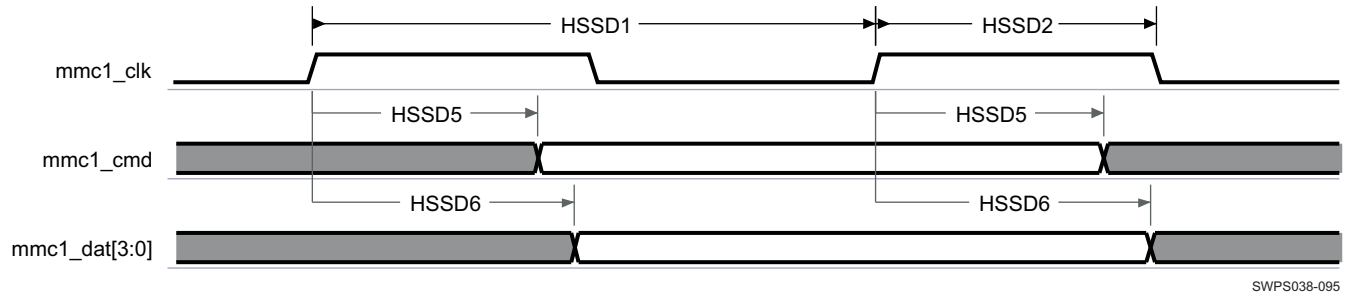
Figure 5-61. MMC1 Interface—High-Speed SD Mode—Data/Command Transmit
