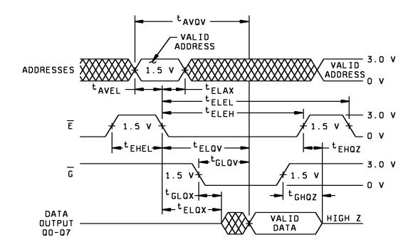
FIGURE 4. Read cycle waveform.
