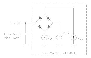
NOTE:  $C_L$  = load capacitance and includes scope and jig capacitance.
