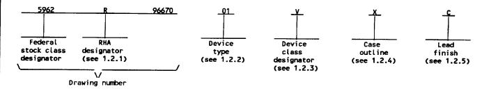
1.2.1 <u>RHA designator</u>. Device class M RHA marked devices shall meet the MIL-I-38535 appendix A specified RHA levels and shall be marked with the appropriate RHA designator. Device classes Q and V RHA marked devices shall meet the MIL-I-38535 specified RHA levels and shall be marked with the appropriate RHA designator. A dash (-) indicates a non-RHA device.
