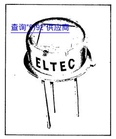
**Model 5192** consists of two physically separate lithium tantalate sensing elements and a FET source follower sealed into a standard TO-5 housing with an optical filter.
