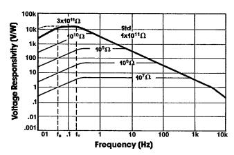
The voltage response of this detector is dependent on the pulse rate or equivalent frequency of input. The frequency response of the detector can be linearized by using a lower value resistor, but at the expense of lower responsivity and a lower D\*. Load resistor values other than the standard 1X10 $^{11}\Omega$  can be specified.
