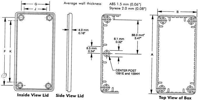
Note: Assembled height = dimension "C" + 4.0 mm (0.16")
