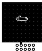
a. 53^\circ\text{C}/\text{W} when mounted on a 1 \text{ in}^2 pad of 2 oz copper
