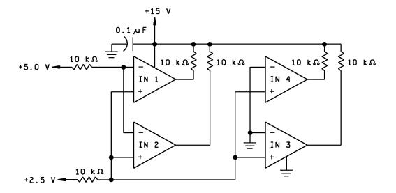
FIGURE 4. Radiation Exposure Circuit.
