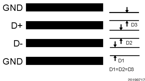
FIGURE 4. Ideal Diode Trace Layout
