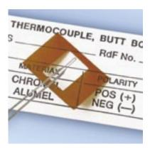
These thermocouples have their free filament supported on a temporary polyimide film carrier. This is a tough, flexible and dimensionally stable material rated at 260°C continuous.
