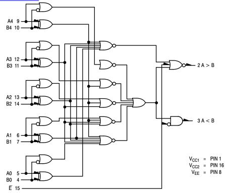
FIGURE 1 – 9-BIT MAGNITUDE COMPARATOR
