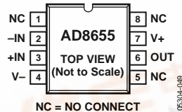
Figure 3. AD8655 8-Lead SOIC (R-8)
