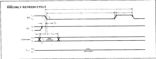
NOTES 1.2 VIH MIN AND VIL MAX ARE REFERENCE LEVELS FOR MEASURING TIMING OF INPUT SIGNALS.
