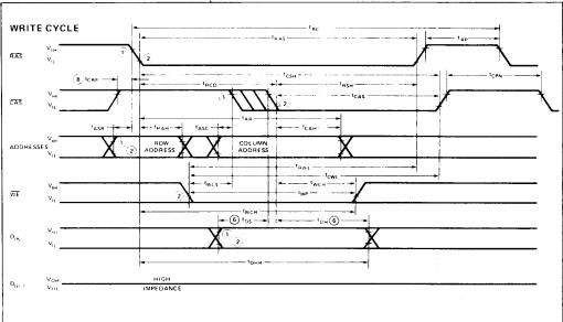
1.2 VIH MIN AND VIL MAX ARE REFERENCE LEVELS FOR MEASURING TIMING OF INPUT SIGNALS
