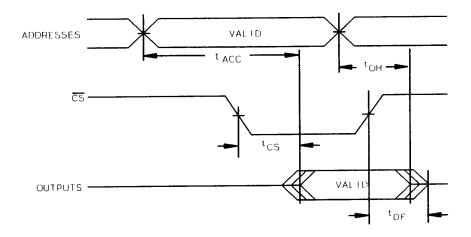
FIGURE 3. AC read timing diagram.
