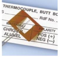
These thermocouples have their free filament supported on a temporary polyimide film carrier. This is a tough, flexible and dimensionally stable material rated at  $260^{\circ}$ C continuous.
