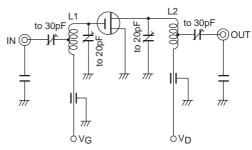
L1: 1.0mm¢ copper wire 10mm¢ 6T, tap: 2.5T from H side L2: 1.0mm¢ copper wire 10mm¢ 7T, tap: 4T from H side
