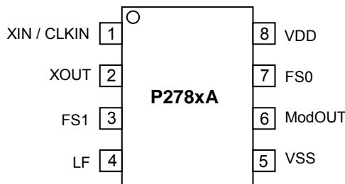
Standard pin Configuration offered in both
