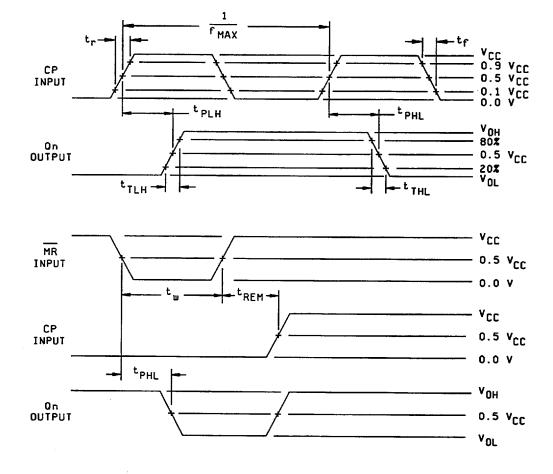
FIGURE 4. Switching waveforms and test circuit.
