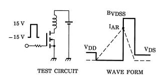
$$\begin{aligned} R_G &= 25~\Omega \\ V_{DD} &= 90~V,~L = 4.59~mH \end{aligned} \qquad E_{AS} &= \frac{1}{2} \cdot L \cdot I^2 \cdot \left( \frac{B_{VDSS}}{B_{VDSS} - V_{DD}} \right) \end{aligned}$$
