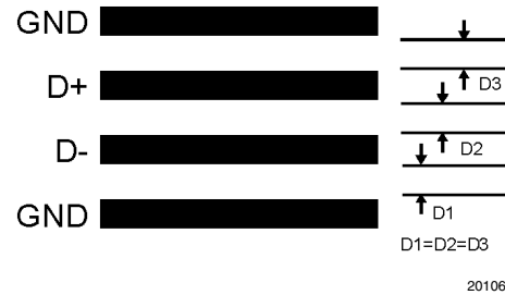
FIGURE 10. Ideal Diode Trace Layout
