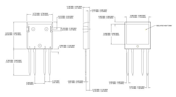
NOTE: Bottom heatsink meets  $2500V_{rms}$  isolation to the other pins.
