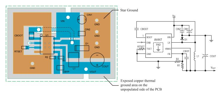
The large star ground area on the populated side of the PCB, shown in the diagram as the GND nodes, supports high current throughput, and allows the VOUT node to be located as close as practical to the A4447 (U1). Thermal conduction from the A4447 is enhanced by direct contact of its exposed thermal pad to the smaller ground area under the A4447. This area is connected by thermal vias to the large copper ground plane on the unpopulated side of the PCB.
