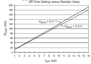
The  $R_{TSET}$  resistor should be not smaller than 7.65 k $\Omega$  ±2% to prevent very short off-times from violating the minimum on-time of the switcher.
