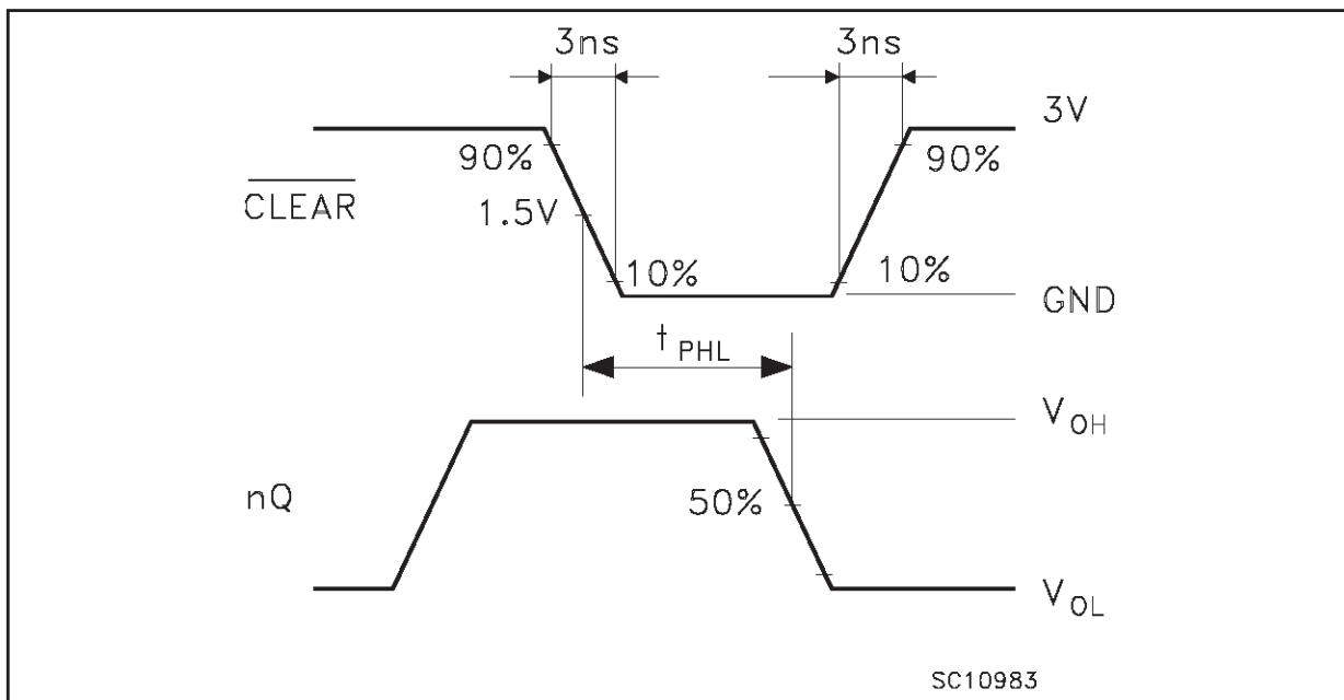
WAVEFORM 3: RECOVERY TIME (f=1MHz; 50% duty cycle)
