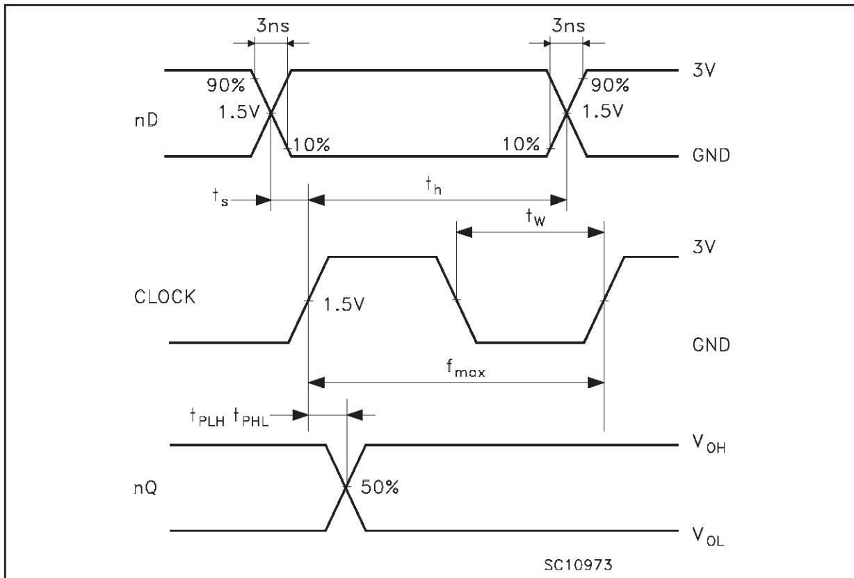
WAVEFORM 2: PROPAGATION DELAYS (f=1MHz; 50% duty cycle)
