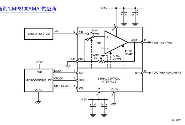
FIGURE 12. Non-Inverting Input Zeroing Function
