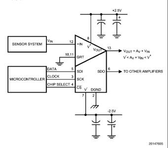
FIGURE 9. Basic Non-Inverting Amplifier
