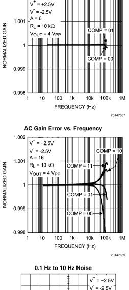
AC Gain Error vs. Frequency
