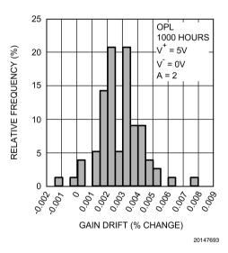
FIGURE 3. OPL Gain Drift, A = 2
