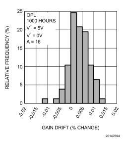
FIGURE 4. OPL Gain Drift, A = 16
