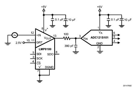
FIGURE 16. Data Acquisition System Using the LMP8100
