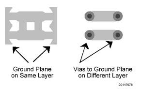
FIGURE 11. GRT Connection Methods
