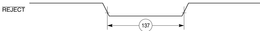
Figure 65. CAM Interface \overline{\text{REJECT}} Timing Diagram
