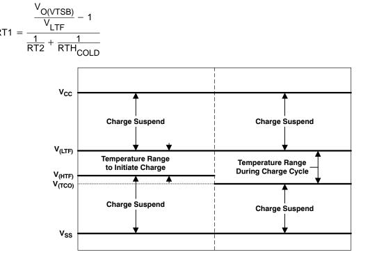
Figure 12. TS Pin Thresholds
