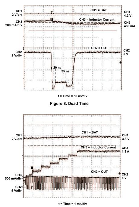
Figure 9. Soft Start Waveforms
