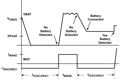
Figure 14. Battery Detect Timing Diagram
