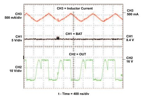
Figure 7. Switching Waveforms in Voltage Regulation Mode
