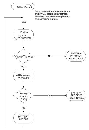
Figure 13. Battery Detection for bq2412x ICs
