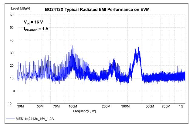
Figure 3. Typical Radiated EMI Performance Measured on EVM
