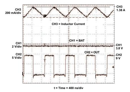
Figure 6. Switching Waveforms in Fast Charge Mode
