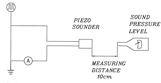
S.P.L. Measuring Circuit Input Signal: 10 Vp-p, 4.8 KHz, square wave Mic: RION S.P.L. meter UC30 or equivalent S.G.: Hewlett Packard 33120A function generator or equivalent
