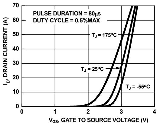
Figure 5. Transfer Characteristics
