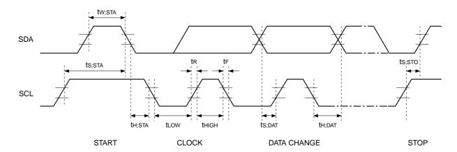
ts;sta = Start setup timetw;sta = Start waiting timeth;sta = Start hold time
