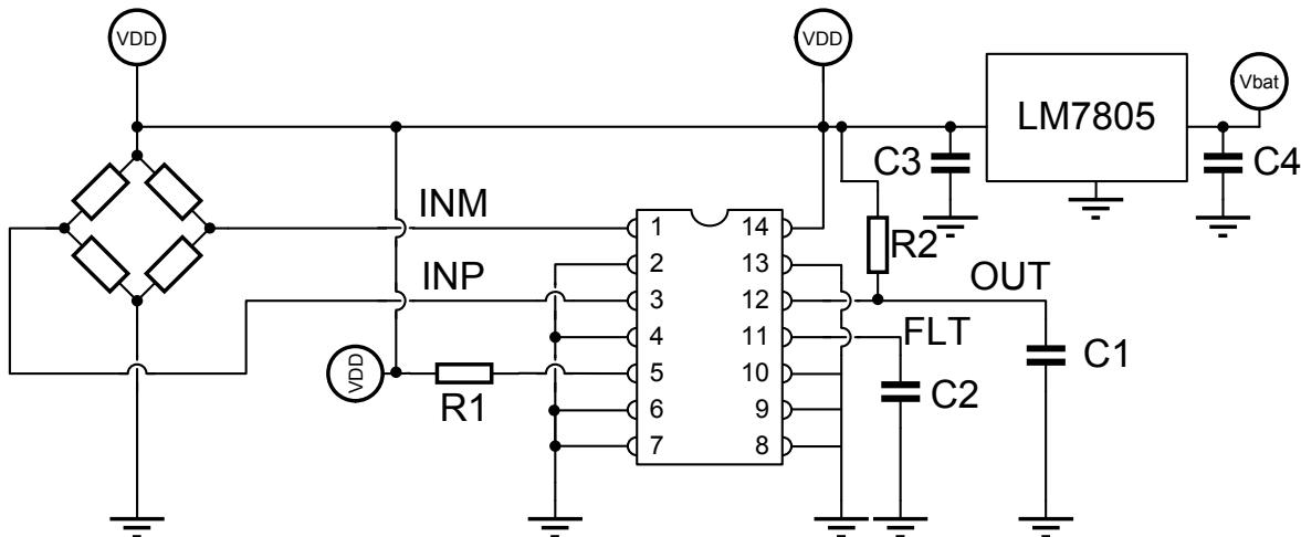
With the use of an external voltage regulator to supply the sensor, the MLX90326 as well as an ADC used for converting the analog output signal, the MLX90326 can be used in a non ratio-metric mode. An example of standard voltage regulator is the LM7805. C1, C2, R1 and R2 are the same as in the ratio-metric application mode. C4 has a typical value of 330nF and C3 of 100nF in this application mode.
