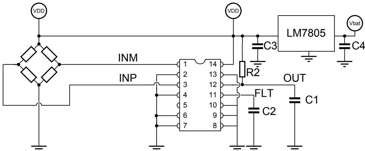
In this application mode the LM7805 generates the supply for the sensor, for the MLX90326 and for an ADC used to convert the analog output signal in a digital value. C1, C2, C3, C4 and R2 are the same as in the non ratio-metric application mode with external temperature sensor.
