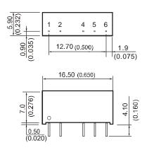
Note: Unit:mm(inch) Pin section:0.50\*0.3mm(0.020\*0.012inch) Pin tolerances:±0.10mm (±0.004inch) Generaltolerances:±0.25mm(±0.010inch)
