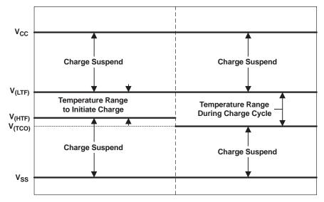
Figure 10. TS Pin Thresholds
