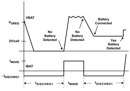
Figure 12. Battery Detect Timing Diagram
