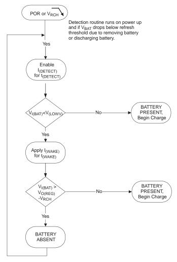
Figure 11. Battery Absent Detection for bq2410x ICs only
