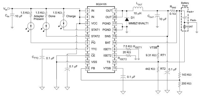
Figure 19. 1-Cell LiFePO4 Application
