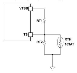
Figure 17. TS Resistor Network
