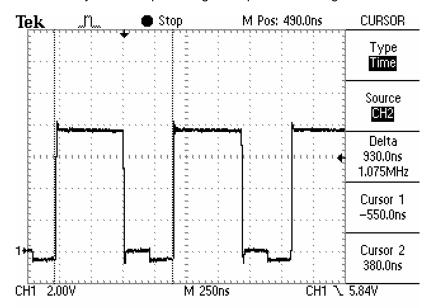
Charge during Voltage Regulation and Approaching Termination: Note that this waveform is similar to the precharge waveform. The difference is that the battery voltage is higher so the duty cycle is slightly higher. The bottom FET stays on longer because there is more of a current load than during precharge; it takes longer for the inductor current to ramp down to the current threshold where the synchronous FET is disabled.
