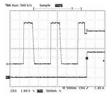
Figure 13. Battery Detection Waveform When a Battery is Inserted
