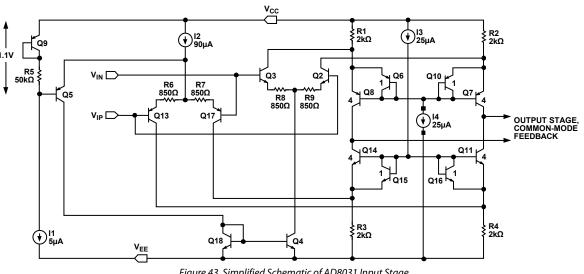
Figure 43. Simplified Schematic of AD8031 Input Stage
