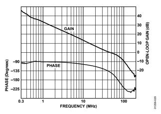
Figure 29. Open-Loop Frequency Response
