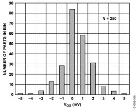
Figure 8. Typical  $V_{OS}$  Distribution @  $V_S = 5 V$
