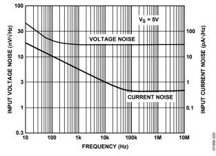
Figure 25. Input Voltage Noise vs. Frequency
