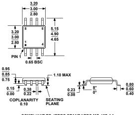
COMPLIANT TO JEDEC STANDARDS MO-187-AA Figure 57. 8-Lead Mini Small Outline Package [MSOP] (RM-8) Dimensions shown in millimeters
