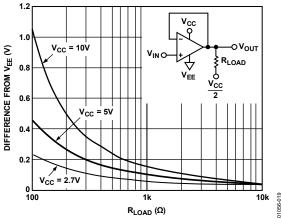
Figure 19. –Output Saturation Voltage vs. R<sub>LOAD</sub> @ –40°C
