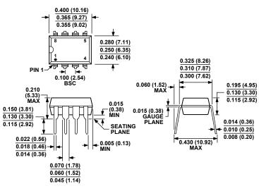
COMPLIANT TO JEDEC STANDARDS MS-001-BA CONTROLLING DIMENSIONS ARE IN INCHES; MILLIMETER DIMENSIONS (IN PARENTHESES) ARE ROUNDED-OFF INCH EQUIVALENTS FOR REFERENCE ONLY AND ARE NOT APPROPRIATE FOR USE IN DESIGN. CORNER LEADS MAY BE CONFIGURED AS WHOLE OR HALF LEADS.
