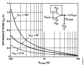
Figure 17. –Output Saturation Voltage vs. R<sub>LOAD</sub> @ +85°C
