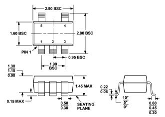
COMPLIANT TO JEDEC STANDARDS MO-178-AA Figure 56. 5-Lead Small Outline Transistor Package [SOT-23] (RJ-5) Dimensions shown in millimeters
