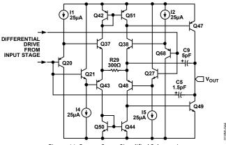
Figure 44. Output Stage Simplified Schematic
