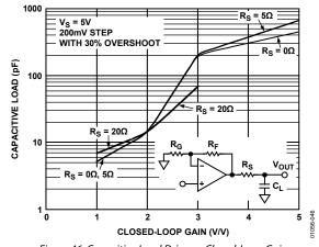
Figure 46. Capacitive Load Drive vs. Closed-Loop Gain
