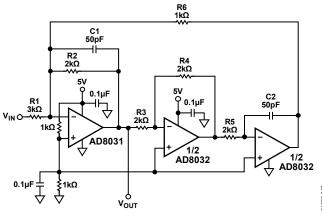
Figure 47. A 2 MHz, Biquad Band-Pass Filter Using AD8031/AD8032
