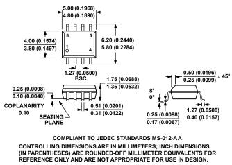
Figure 55. 8-Lead Standard Small Outline Package [SOIC\_N] Narrow Body (R-8) Dimensions shown in millimeters and (inches) 060506-A
