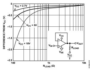
Figure 15. +Output Saturation Voltage vs. RLOAD @ +25°C
