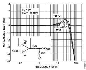
Figure 27. Closed-Loop Gain vs. Temperature
